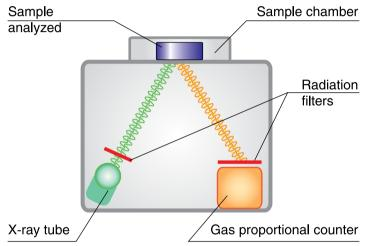
X-ray fluorescence energy dispersive sulfur analyzer ASE-2 is used for the measurement of mass concentration of the sulfur in unleaded gasoline, diesel oil, crude oil, kerosene, petroleum residues, lubricating oil, hydraulic oil, jet engine fuel and other types of cutter oil.
