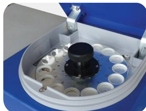
Changer is able to carry solid, liquid or powder samples
