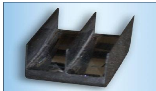
X-ray interferometer. Si(220), 2d=0,384 nm
