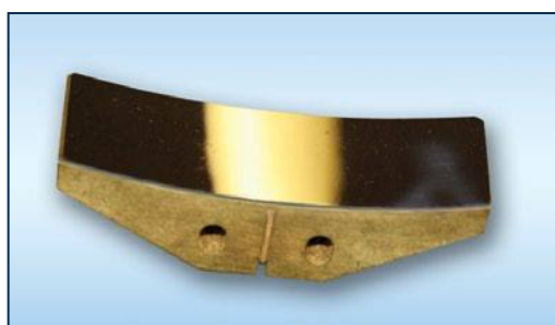
Johann cylindrical analyzer. InSb(111), 2d=0,748 nm
