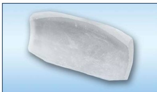
Toroidal monochromator. R1=150 , R2=75 , LiF(200), 2d=0,403 nm
