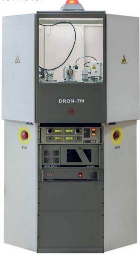
DRON-7M X-ray diffractioneter is capable to solve a wide variety of tasks for powder diffraction analysis. Independent control of  $2\theta$  and  $\theta$  movements allows research of single crystals.
