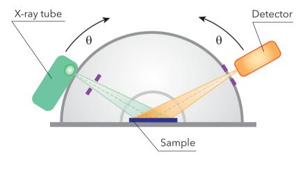
DRON-8/8T X-ray general purpose diffractometer with vertical  $\theta$ - $\theta$  goniometer and horizontal sample plane enables to perform X-ray diffraction analysis of phase composition, structural state and orientation of wide range of crystalline objects with different shape and size.
