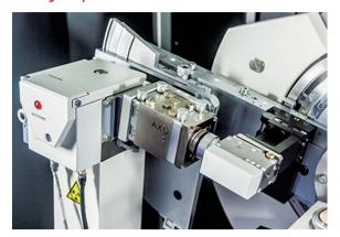
**One-dimensional parabolic mirror** for DRON-7, DRON-8/8T. Converts a divergent primary beam to a parallel one, makes it monochromatic and enhances intensity.
