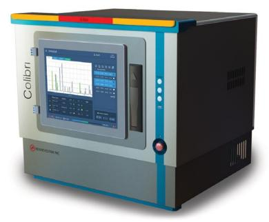
Vertical  $\theta {-} \theta$  goniometer of unique design with horizontal sample position
