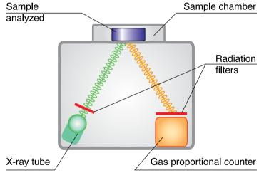
X-ray fluorescence energy dispersive sulfur analyzer ASE-3 is used for the measurement of mass concentration of the sulfur in unleaded gasoline, diesel oil, crude oil, kerosene, petroleum residues, lubricating oil, hydraulic oil, jet engine fuel and other types of cutter oil.
