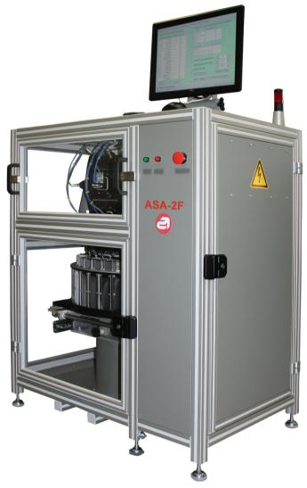
Diamond sorting machine is designed for automatic diamonds classification by shape and its sorting in 10 groups.
